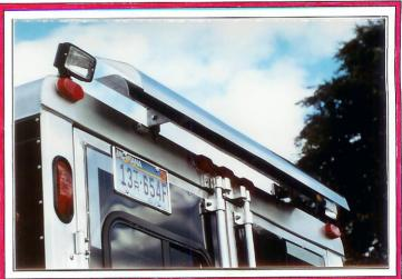
Are your horses and stock covered with *dust, road grime, rain, and snow* from being transported in your trailer? The <u>See II Air Foil</u> reduces this problem and keeps the rear of your trailer clean. By capturing and shooting <u>two streams of clean air</u> down the back of the trailer, the rear of the trailer and lights are kept clean, and dust, road grime, rain and snow is not allowed to reach your horses.
