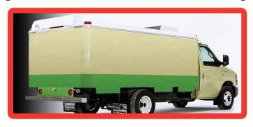
Have you always hated the way your trucks look when the backs are covered with dust, snow, and road grime? The See II Air Foil reduces the problem of keeping the rear of the truck clean, by capturing and shooting two streams of clean air down the back of the truck. As a result the truck and lights remain clean from dust, snow, and road grime buildup for a longer period of time.
